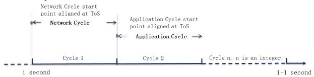
Figure 10 – Top-of-Second Alignment of Application Cycle and Network Cycle
