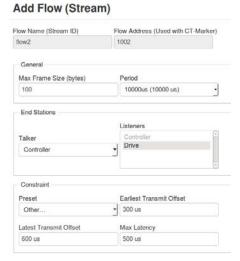
Figure 2 – Add TSN Streams by Specifying Constrains in DE-CNC
