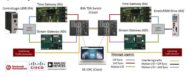
Figure 1 – Testbed of CIP Motion over TSN
